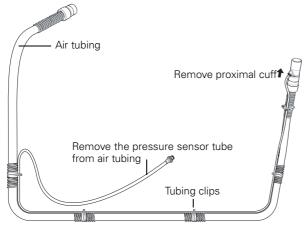
Figure 19: Air tubing assembly removed for cleaning
